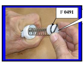
Install **O-rings** onto plunger
