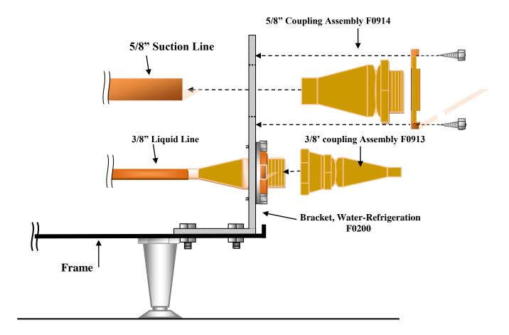
NOTE: The assemblies with part numbers F0913 and F0914 include male and female halves as well as the hold-down washer.
