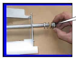
Step 5: Install spring seal **F0355**
